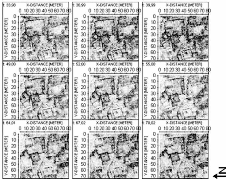
Fig. 4: Time slices diagram of GPR equal amplitude echoes at the central part of the Eastern residential area (cf. also Fig. 2. A)
