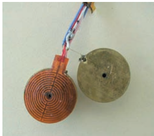
Figure 2: Spherically shaped Melting Probe with commercial Kapton heating foil.
