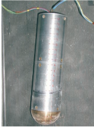
Figure 3: Picture of the Melting Probe after the test. The black line marks the penetration depth reached during the melt down.
