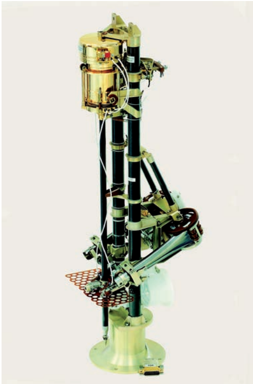
Figure 1: The MUPUS penetrator in its stowed configuration, FS model.
