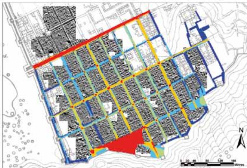
Fig. 5: Visibility Graph Analysis of the network of streets (The colour scale expresses the values of visual connectivity.)
