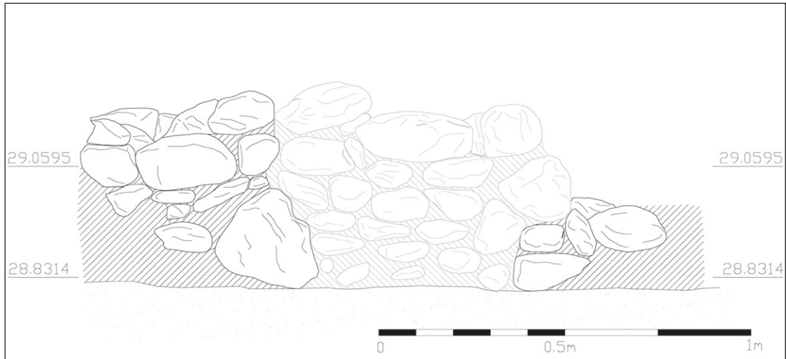
Fig. 5.3 View of the closed gap in the northern wall of room 18 (black: original wall; grey: filled in part) (plan: M. Börner, St. Grasböck)
