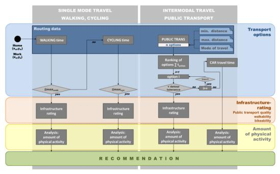
Figure 1: General scheme of the analysis of intermodal routing options for the selection of healthy routes to/from work.
