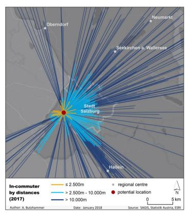
Figure 4: Visualization of commutes for a potential business location. The relation is classified according to the network-based distance in order to derive potential users for the different modes of transport.
