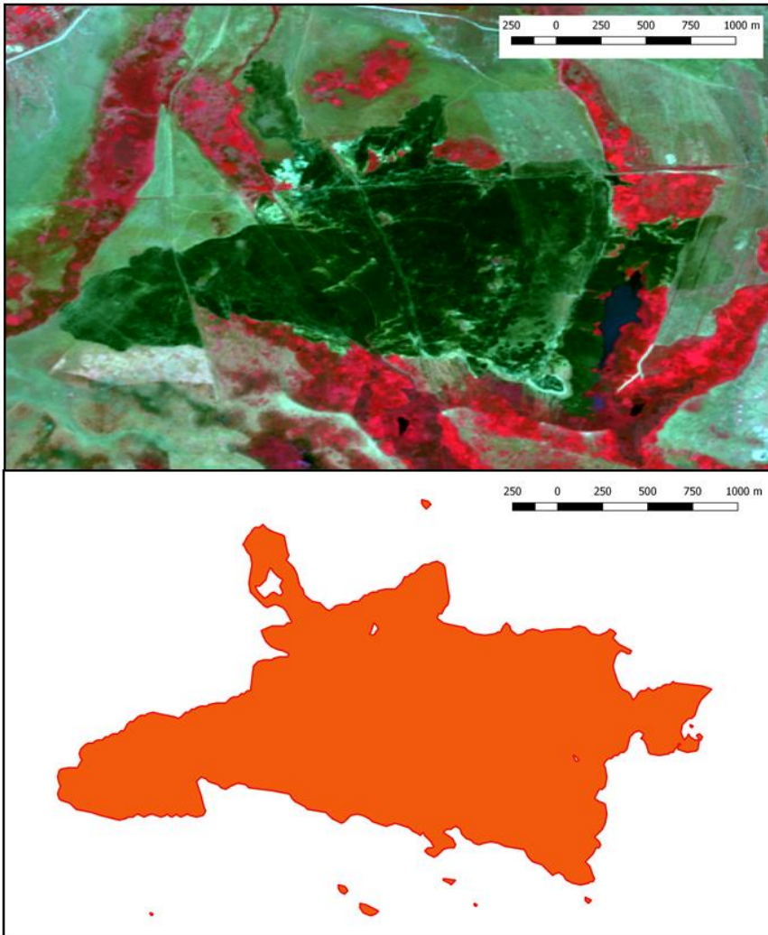
Figure 6: Post-fire false-colour image (bands 8, 4, 3) and Burned Area Map for EMSR230. The blackened area represents charred vegetation.
