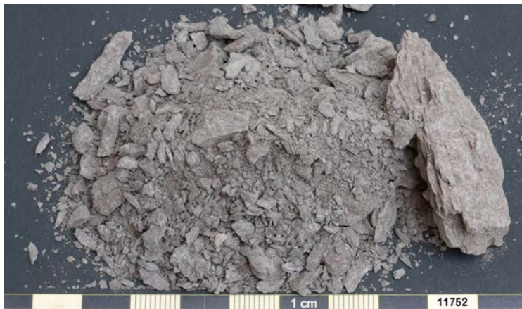
Fig. 3.41 Likir. Sample 11752. Sample colour (after Munsell): Dry 10YR 5/1 grey. Semi-dry 10YR 4/1 dark grey.
