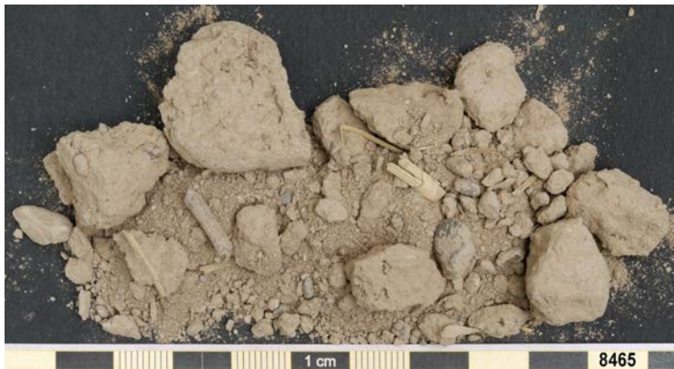
Fig. 3.22 Basgo. Sample 8465. Sample colour (after Munsell): Dry 10YR 7/2 light grey. Semi-dry 10YR 5/3 brown.
