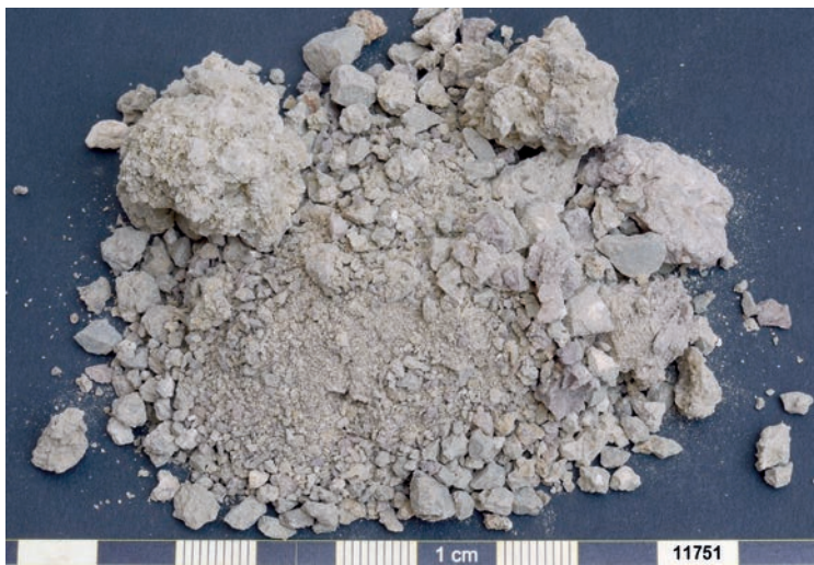
Fig. 3.39 Basgo. Sample 11751. Sample colour (after Munsell): Dry 10YR 7/2 light grey. Semi-dry 10YR 6/3 pale brown.
