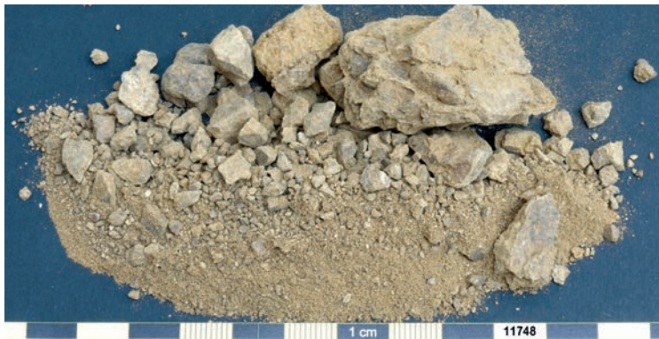
Fig. 3.28 Tunlung. Sample 11748. Sample colour (after Munsell): Dry10YR 7/6 yellow. Semi-dry 10YR 5/6 yellowish brown.
