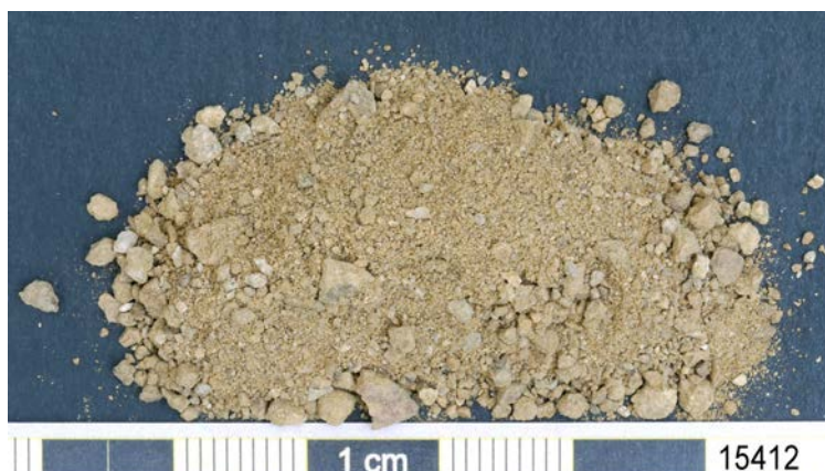
Fig. 3.35 Tunlung. Sample 15412. Sample colour (after Munsell): Dry 10YR 7/6 yellow. Semi-dry 10YR 5/6 yellowish brown.
