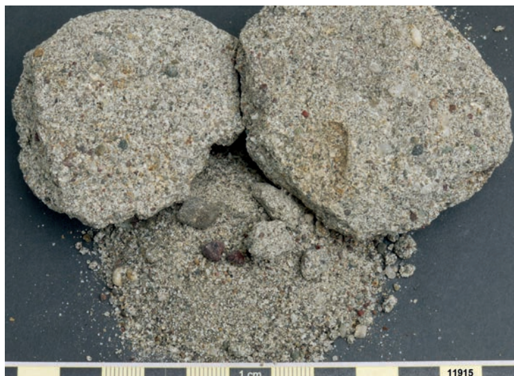
Fig. 3.20 Basgo. Sample 11915. Sample colour (after Munsell): Dry 10YR (6)7/1 light grey. Semi-dry 10YR 4/1 dark grey.
