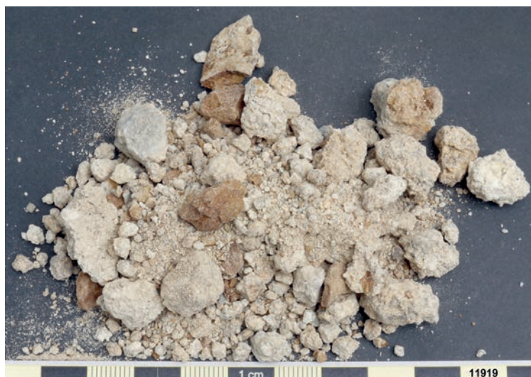
Fig. 3.37 Tunlung. Sample 11919. Sample colour (after Munsell): Dry 10YR 8/1 white. Semi-dry 10YR 8/2 very pale brown.
