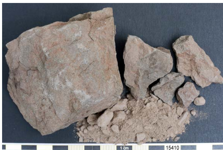
Fig. 3.19 Basgo. Sample 15410. Sample colour (after Munsell): Dry 10YR 6/2 light brownish grey. Semi-dry 10YR 4/2 dark greyish brown.
