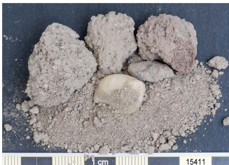
Fig. 3.21 Basgo. Sample 15411. Sample colour (after Munsell): Dry 10YR 6/2 light brownish grey. Semi-dry 10YR 4/2 dark greyish brown.
