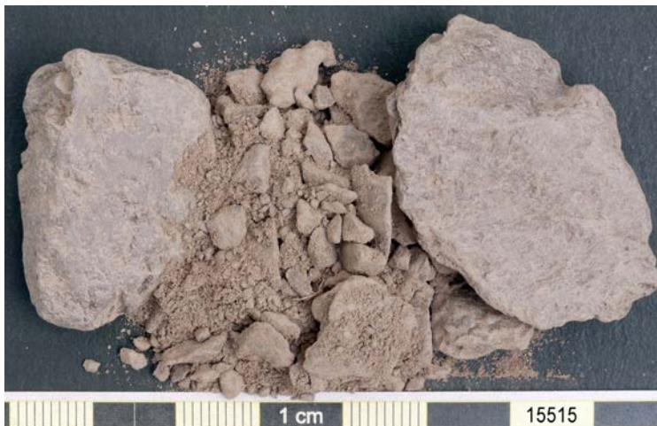
Fig. 3.38 Basgo. Sample 15515. Sample colour (after Munsell): Dry 10YR 8/1 white. Semi-dry 10YR 8/2 very pale brown.
