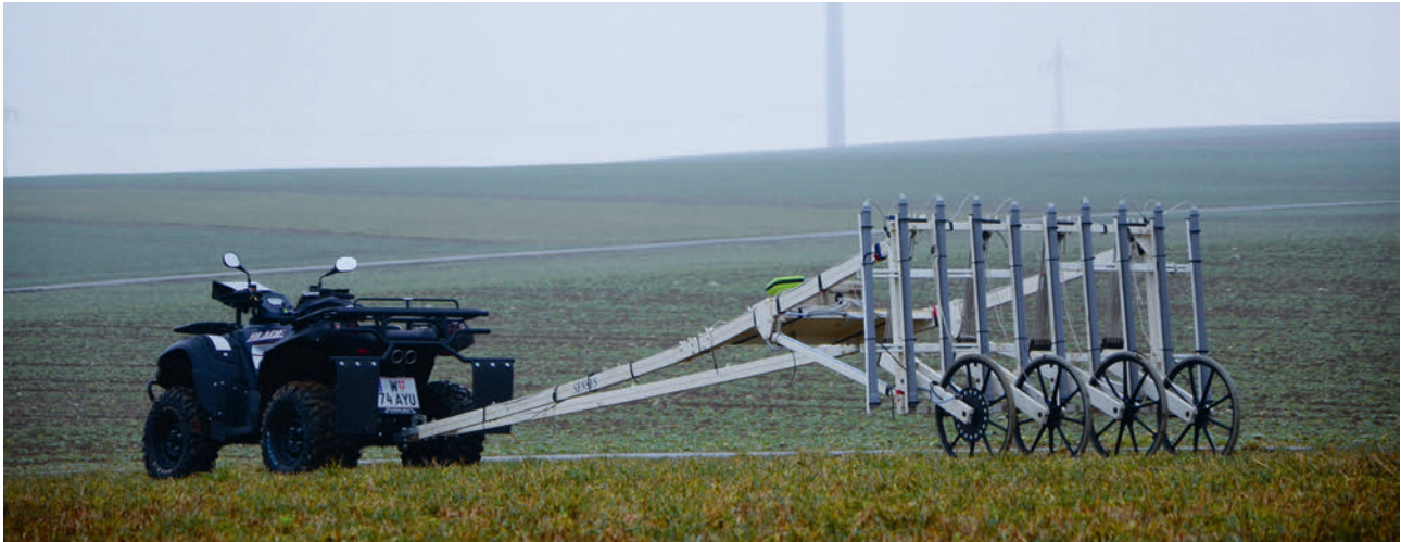
Fig. 2. Motorised magnetic prospecting. The ten Foerster FEREX CON650 gradiometer probes are mounted on the cart, which is towed by an ATV. The wheels are independently suspended (LBI ArchPro, M. Kucera).
