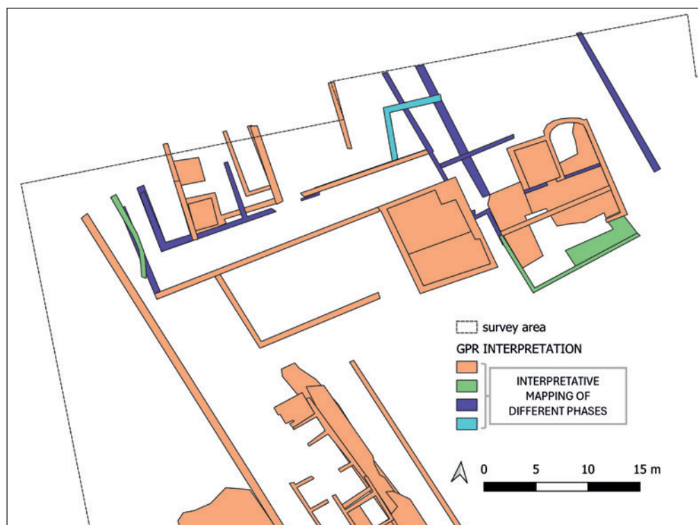
Fig. 17. 'Phasing map' of wall structures in the northern area; the classification by phases, indicated by different colours, does not correspond to a specific chronology; in fact, it would be very arduous to reconstruct even a mere relative chronology if working only with GPR data (Graphics: V. Poscetti).
