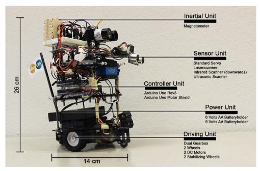
Figure 2: Configuration and dimensions of the SLAM robot.
