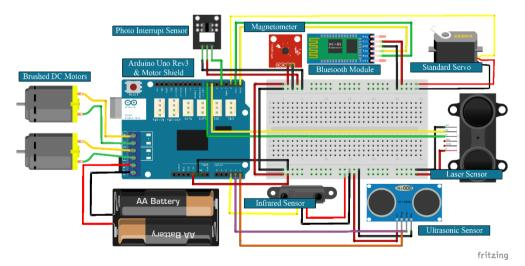
Figure 3: Wiring scheme for the SLAM robot.
