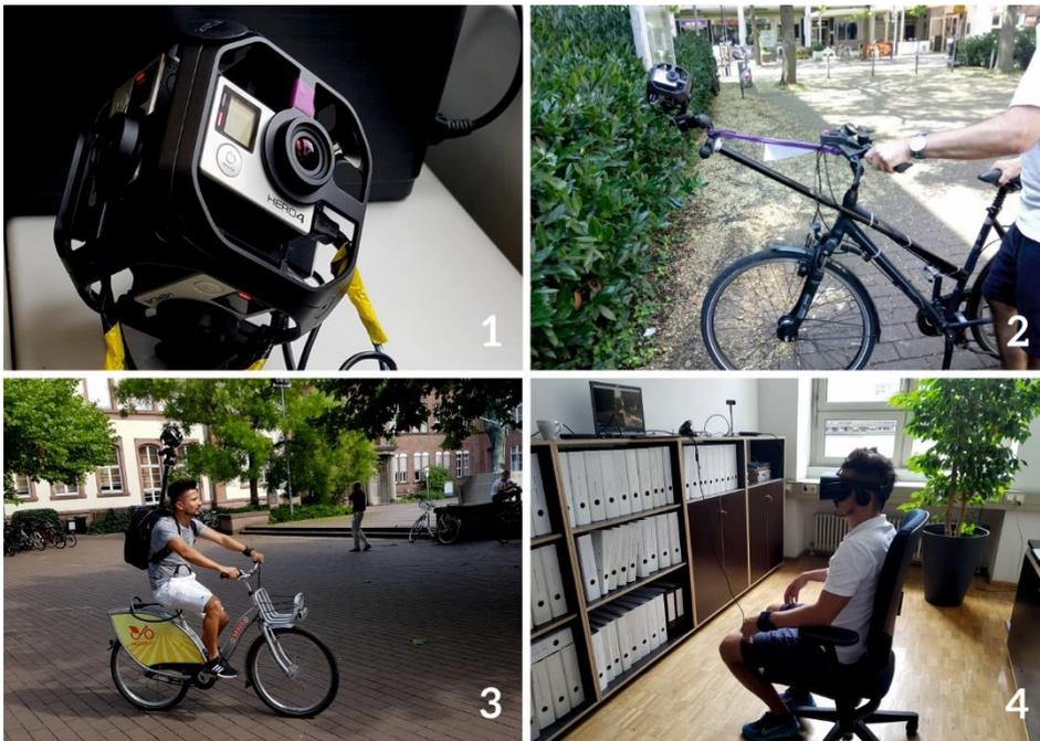
**Figure 1:** (1) The Omni-Rig, with its six synchronized action cams for creating spherical videos. (2) Test drives in the so-called 'cantilever mode' and (3) in the 'Streetview mode'. (4) The composite video can now be viewed on the Oculus and used as an audio-visual test environment for biostatistical monitoring.
